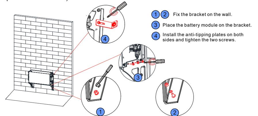
Figure 4-10: Fix the bracket to the wall
