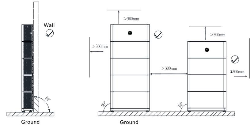
Figure 4-2: Floor-mounted installation
