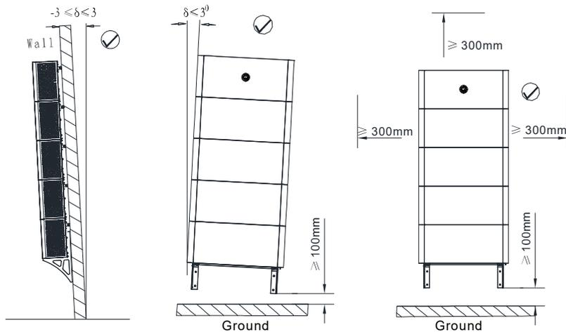
Figure 4-1: Wall-mounted installation
