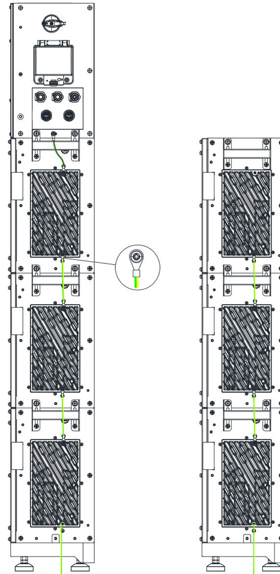
Figure 4-23: Two-column installation
